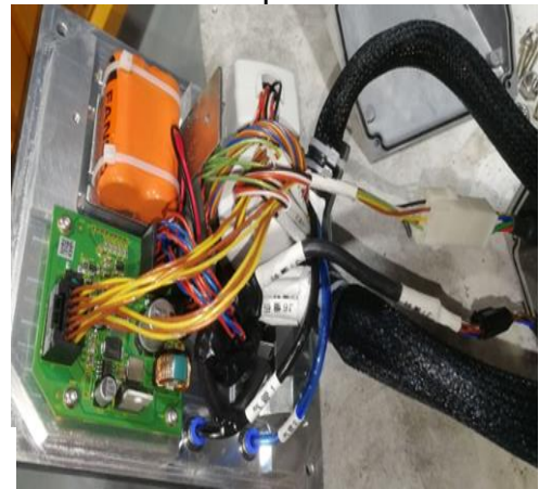
Fig. 6.3 Fixing of Internal Battery
