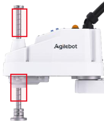
Fig. 6.4 Diagram for Greasing Area on Screw Splines
